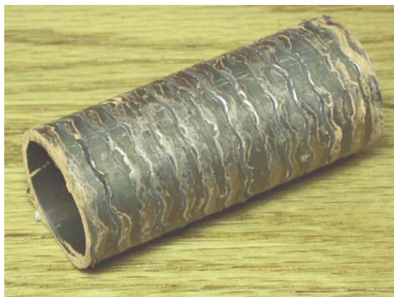
Figure #8 - 409SS fins / SB423 NO8825 after 48 hours
