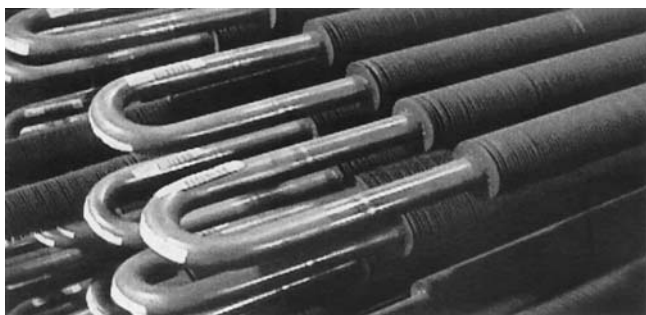
Figure 6 OTSG alloy 825 heat exchanger tubes and stainless steel fins.
