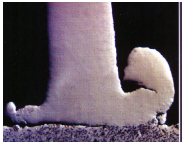
Figure 4; The braze finning process (left) creates a very effective heat transfer surface, while minimizing the impact on the tube integrity.
